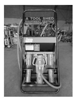
Kit includes: Cart, P-55 Post Driver with Control Handle, 2" 2  $\frac{1}{2}$ " 3" 3  $\frac{1}{2}$ " Post Adaptors, Channel Post Adaptor, Air Oiler/Water Trap with 12' Hose, 1 quart of Oil for the Oiler and two  $\frac{1}{2}$ -13 x 1  $\frac{1}{2}$ " bolts with compression washers.
