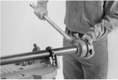
Figure 3 – Sliding Threader on Pipe
